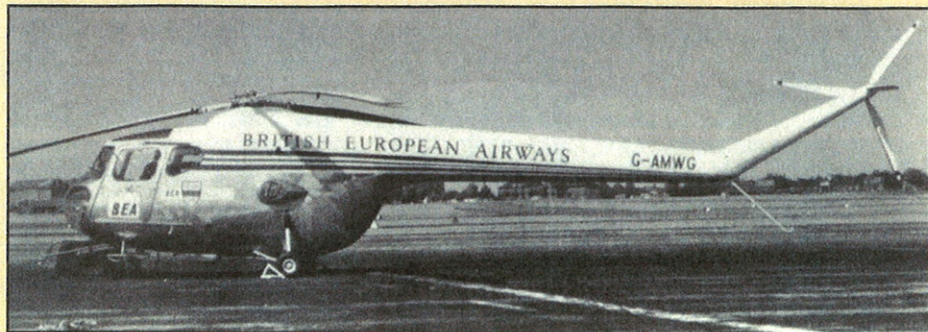
Below: The diminutive 3-passenger Bristol 171 Sycamore was a slight improvement over BEA's Sikorsky S-51s, and went into service in 1953. With a maximum speed of 120 mph it offered only a slight advantage over trains when covering its max. 430-mile operating range. Bristol was eventually taken over by Westland.
